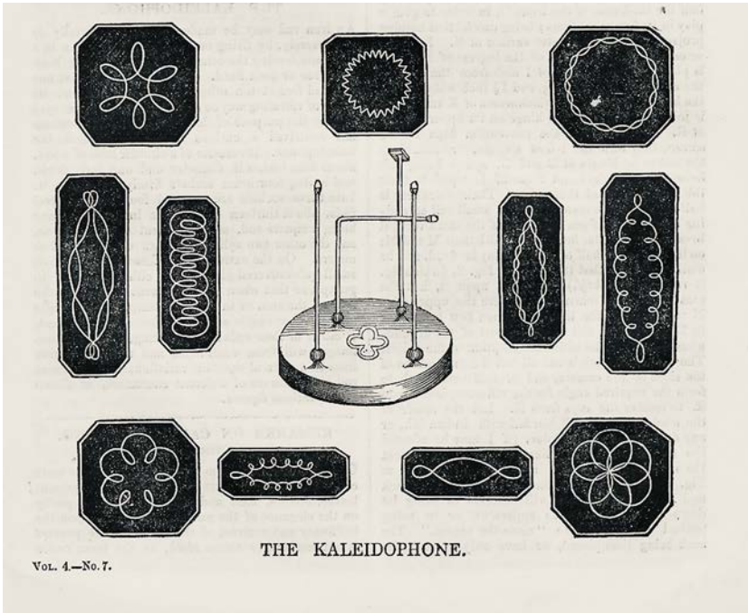
FIGURE 4. Charles Wheatstone's kaleidophone (1827), advertised on the frontispiece of the Magazine of Science on May 14, 1842, showing the apparatus (center) encircled by examples of the variety of its resulting vibrational patterns. Credit: Cambridge University Library.
