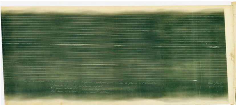
FIGURE 9. Martinville's test sheet setting vocal inflection alongside tuning fork vibration: "Acoustic effect of declamation with simultaneous tuning fork to show the inflection of the intonation ... April 17, 1860" (Bibliothèque de l'Institut de France, MS 2935, no. 89095). From his talk "Fixation et transcription du chant" (1860): https://www.firstsounds.org/publications/facsimiles/FirstSounds_Facsimile_05.pdf .
